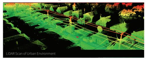
In preparation for each project, the utility contractor surveys utility poles and their transformer units to identify access points in a given area where the smart grid mesh would be implemented. Each access point serves as a local receiver of smart meter data transmitted over existing cellular networks. There are roughly 4,000 smart meters for every access point. The information is then collected through a network of relay transmitters.
